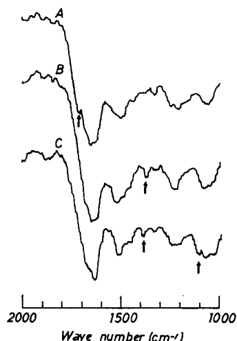
Fig. 8. Reflection infrared spectra of free and aggregated cells. A and B show the spectra of free cells washed with HCl solution (pH 3) and with NaOH solution (pH 8), respectively; C is the spectrum of cells aggregated with TGCI at pH 8 and washed with HCl solution (pH 3).
